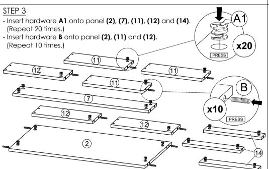
\* Ensure the arrows on hardware A1 point towards mounting positions.
