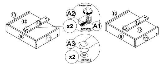
\* In this step hardware A1 and A2 are pre-inserted.
