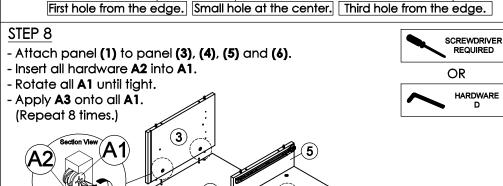
\* In this step hardware A1, A2 and B are pre-inserted.
