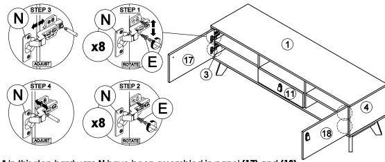
\* In this step hardware N have been assembled in panel (17) and (18).
