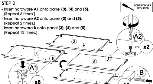
\* Ensure the arrows on hardware A1 point towards mounting positions.
