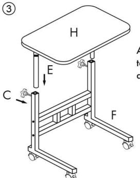
Attach the assembled part 2 to part 1 at the desired height and tighten the butterfly knobs.
