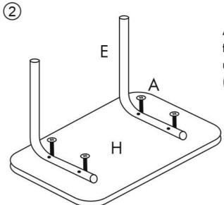
Align E - the elbows on H the desktop board and install using A - the flat head screw (short).
