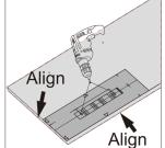
Install the door fittings and affix onto the door panel using 4x screws.
