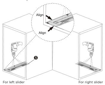
Install the sliders and affix onto the cabinet floor using 12x screws.
