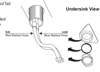
2 Fit Rubber Ring into groove on the mixer base.
