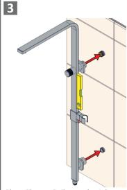
Place Shower Rail onto the Adaptor and Wall Mounting Bracket.
