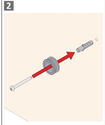
Screw Mounting Bracket into wall.
