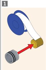
Apply Teflon Tape to the Wall Thread and attach the Shower Adaptor.
