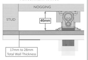
Range from the Nogging face to the Stud Face is 46mm as shown.
