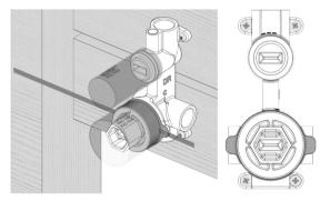
Check Lugs (Highlighted in ORANGE) are Flush with Front of Stud.
