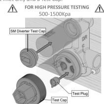
For high pressure testing of pipes, remove Test Cap and add another Test Plug into the Cold Inlet.
