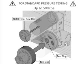
SwitchMix comes pre-installed with a Test Plug in the Hot Inlet only and a Test Cap.
