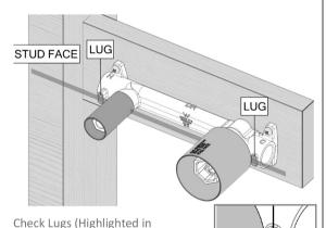
1 Screw the Mixer Breach onto Nogging to dimensions shown in adjustment range.
