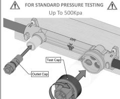
SwitchMix comes pre-installed with a Test Plug in the Hot Inlet only and a Test Cap.
