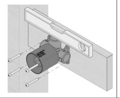
Create a 50mm diameter hole in the cement sheet or Plasterboard.
