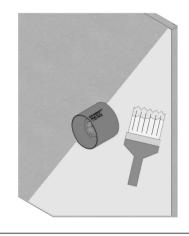
After Tiling use Knife to Trim Waterproofing Sleeve flush to Tile face.
