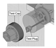
For high pressure testing of pipes, remove Test Cap and add another Test Plug into the Cold Inlet.
