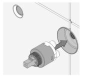
Add grease or soap to Cartridge Legs. Push Cartridge gently Into Body. Ensure correct orientation.
