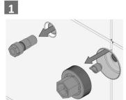
Remove Test Caps with a flat head screwdriver or spanner.
