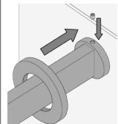
Tighten Grub Srew securing spout to addaptor.
