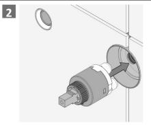
Add grease or soap to Cartridge Legs. Push Cartridge gently Into Body. Ensure correct orientation.
