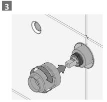
Firmly fasten Cartridge Sleeve to Mixer Body using a shifting spanner.
