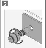
Align outlet hole in wall with outlet hole in Dress Plate.
