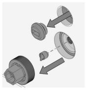
Remove Test Caps with a flat head screwdriver or spanner.
