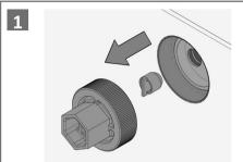
Remove Test Cap using a Flat Head Screw Driver or spanner.
