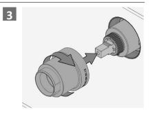
Firmly fasten Cartridge Sleeve to Mixer Body using a shifting spanner.
