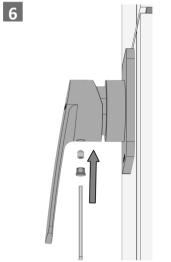
Tighten Grub Screw and push in Cap to secure handle.
