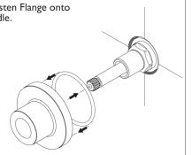
Fit Handle Hub to Spindle and fasten with the Grub Screw using the Allen Key provided. Screw the Handle Pin into the Handle Hub
