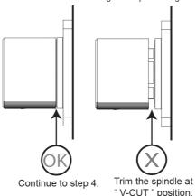
Turn the spindle Anti-Clockwise until the cartridge is set to OFF position.
