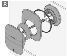
Push Dress plate onto Cartridge and tighten Mixer Dome into place.
