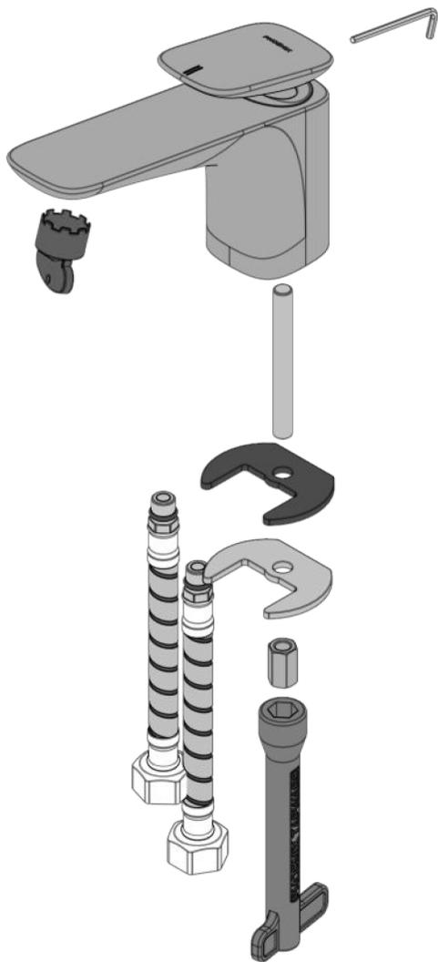
**1** Cut a mounting hole 35mm in diameter. There must be a minimum 12mm clearance around the hole.
