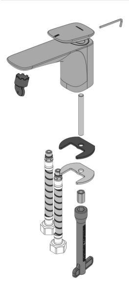
Cut a mounting hole 35mm in diameter. There must be a minimum 12mm clearance around the hole.
