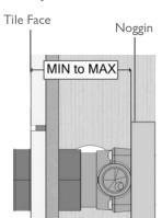
MIN: 68mm MAX: 80mm Screw the Mixer Breach onto Nogging. Ensure that the mixer body centres are level.
