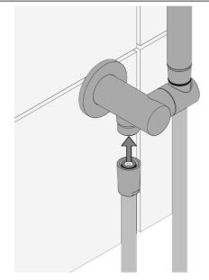
Connect hose and Handpiece. Turn on and check for leaks. 3
