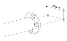
For fixing to brick walls with hard plaster or ceramic tiled surface:
