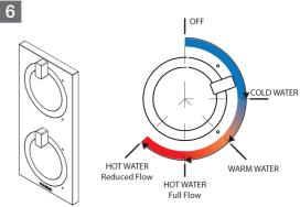
The ORTHO mixer range uses Progressive Cartridge Technology. Rotate the handle clockwise. First position is COLD water only Second position mixes hot and cold water for WARM water. Third poistion is HOT water only
