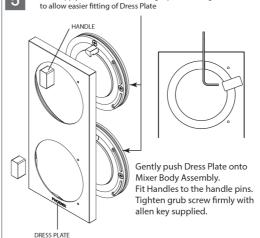
Note: Apply a smear of dishwashing liquid to O Rings
