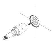
2 Fit Fibre Washer around the Spindle and then firmly fasten the Bonnet onto the Spindle using a spanner.
