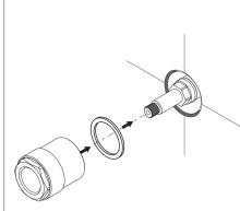
Fit O-Ring to the groove in the rear of the Dress Plate.
