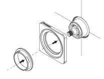
Turn the spindle clockwise until the cartridge is set to OFF position.
