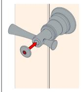
Push temperature indicator caps onto handles as shown.
