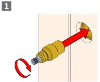
Screw Cartridge Body into recess till Catridge Seat meets a physical stop.
