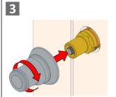
Screw Flange to the Bonnet until flush with wall.
