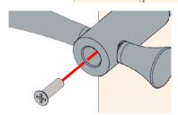
Fit Handle Assembly over spline. Ensuring Handles are level.
