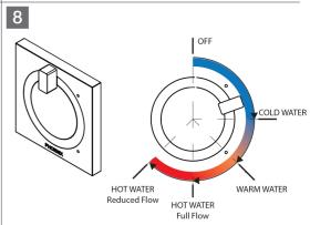
The ORTHO mixer range uses Progressive Cartridge Technology. Rotate the handle clockwise. First position is COLD water only Second position mixes hot and cold water for WARM water. Third poistion is HOT water only
