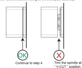
Turn the spindle Anti-Clockwise until the cartridge is set to OFF position.
