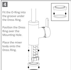
Underneath the Mounting Hole, feed the Rubber Mounting Gasket then the Mounting Plate onto the Threaded Rod.
