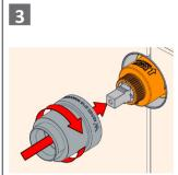
Fasten Cartridge Sleeve to Mixer Body using a shifting spanner.
