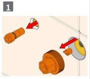
Remove Test Caps with a flat blade screwdriver or spanner.
