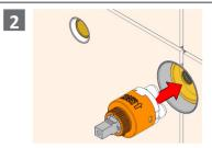
Add grease or soap to Cartridge Legs. Push Cartridge gently Into Body. Ensure correct orientation.
