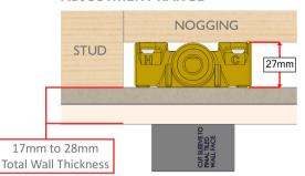
Range from the Nogging face to the Stud Face is 27mm as shown.
