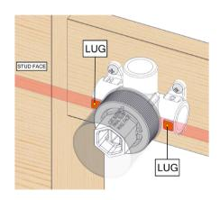
Check Lugs (Highlighted in ORANGE) are Flush with Front of Stud.
