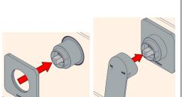
3 Create a 50mm diameter hole in the cement sheet or Plasterboard.
