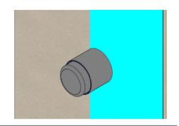
Tighten Grub Screw and push in Cap to secure handle.
