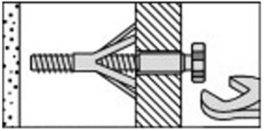
4. Cavity Fixing Heavy Duty Wall Plug
