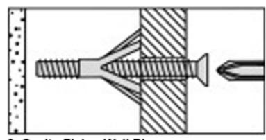
Cavity Fixing Wall Plug
