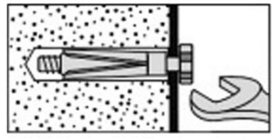
6. Shield Anchor Wall Plug Heavy Loads For use with concrete or brick walls, or for use with heavier loads such as TV & WIFI speakers and satelite dishes, etc.
