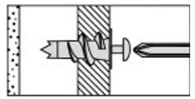
Plasterboard Wall Plug For use when attaching light loads onto plasterboard partitions.
