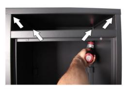
Step 4: Install the top lid. Make sure that the double folded edge is on the front and the single folded edge closes off the rear board. Then screw the lid with the side boards at the marked places.
