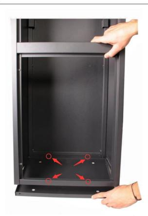
Step 5: Install the bottom panel. Tilt the box backwards on a soft surface. Insert the bottom panel. Make sure that the clips on the side panels enclose the edges of the bottom board. Push the bottom and you will hear a click. Then screw the bottom to the rear board at the marked point with a self-tapping screw.
