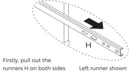
runners H on both sides of the unit to extend about 10cm to 15cm out.
