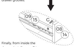
drawer, install screw G to thread through the indicated hole on runner H.
