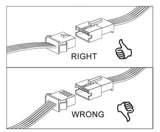
Check the facing of the connectors and ensure that they are aligned correctly.
