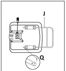
Slide the footrest frame (J) into the footrest plate holders and secure the footrest assembly with screws (Q).
