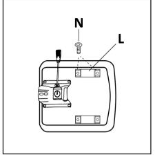
Attach the two footrest plate holders (L) to the seat cushion (E) with screws (N).
