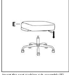
Insert the seat cushion sub-assembly (E) into the gas lift (H).
