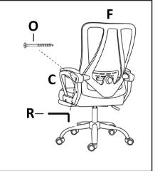
Attach the backrest (F) to the armrests (C) with screws O.
