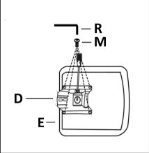
Attach the seat plate (D) beneath the seat cushion (E) with screws (M).
