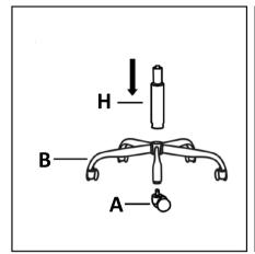
Attach the castor wheels (A) to the 5-prong base (B). Then insert the gas lift (H) into the centre hole of the base as shown.
