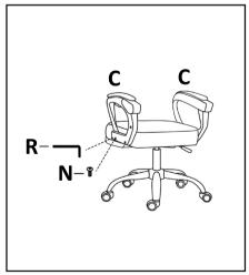
Install the two armrests (C) to the seat cushion as shown with screws (N).
