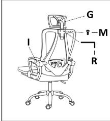
Attach the headrest (G) to the backrest (F) with screws (M). Finally, attach the armrest covers (I) to the armrests (C).
