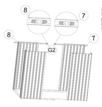
NOTE: Ensure that the positioning of G2 is of the correct facing.
