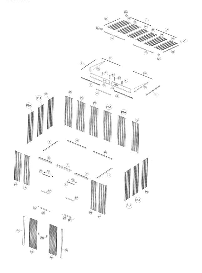
Assemble the base bars (1 to 4L) with screws F1. Next, place the entrance taper channel (5) on top of the bars (3L and 3R). Secure with screws F1 to the base as shown. Ensure that the base bar assembly is a perfect rectangle.
