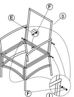
Attach D to arms of A and B using 2 bolts (H) and 2 washers (F). Next, secure bottom of D to back of seat using one bolt (E) and one washer (F).
