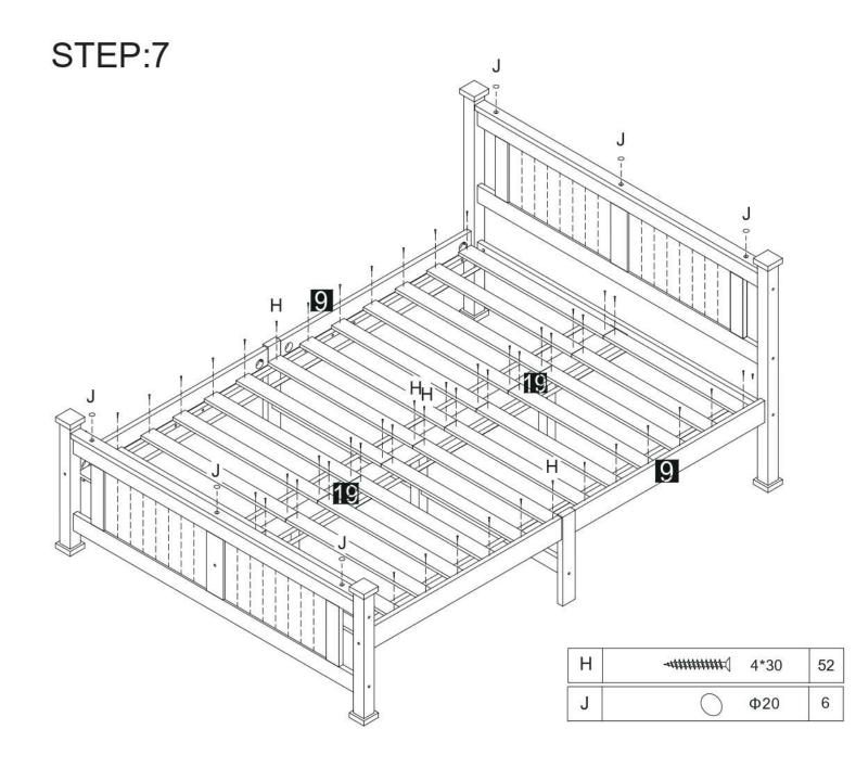
Note:1 Do Not use power tools! Tighten all screw H to fix all bed slats
