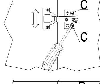
3)Height adjustment: Lossen screw C, adjust door height and lock screw C.
