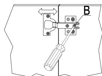
2)Depth adjustment: Loosen screw B, push hinge arm forwards or backwards, and then lock screw B.
