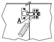
1)Side to side adjustment: Adjust the clearance between door and cabinet by turning screw A.
