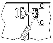
3)Height adjustment: Lossen screw C, adjust door height and lock screw C.
