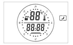
When the heater is in operation, press  $\bigcup_I \bigoplus$  for 3 seconds. The child lock function will be turned on and the screen will display  $\bigoplus$ . In this mode, the child lock function cannot be released.
