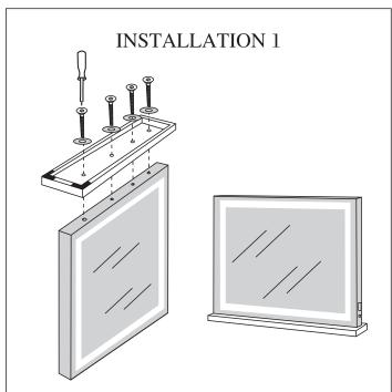
1. Align the holes in the mirror base and bottom, then tighten the screws.
