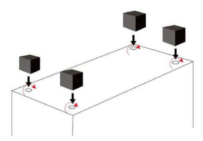
Warning: Make sure four legs are fixed on tightly to prevent from falling off afterwards.
