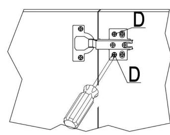
4)Fixed: After adjustment, lock screw D. Make the hinge can't move. 8
