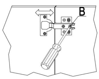
2)Depth adjustment: Loosen screw B, push hinge arm forwards or backwards, and then lock screw B.
