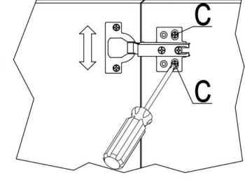
3)Height adjustment: Lossen screw C, adjust door height and lock screw C.
