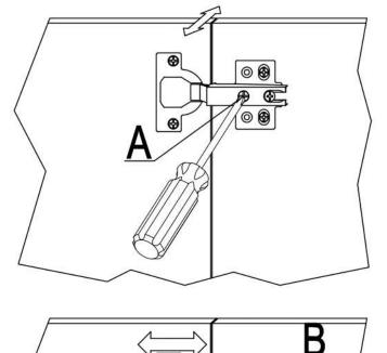
1)Side to side adjustment: Adjust the clearance between door and cabinet by turning screw A.
