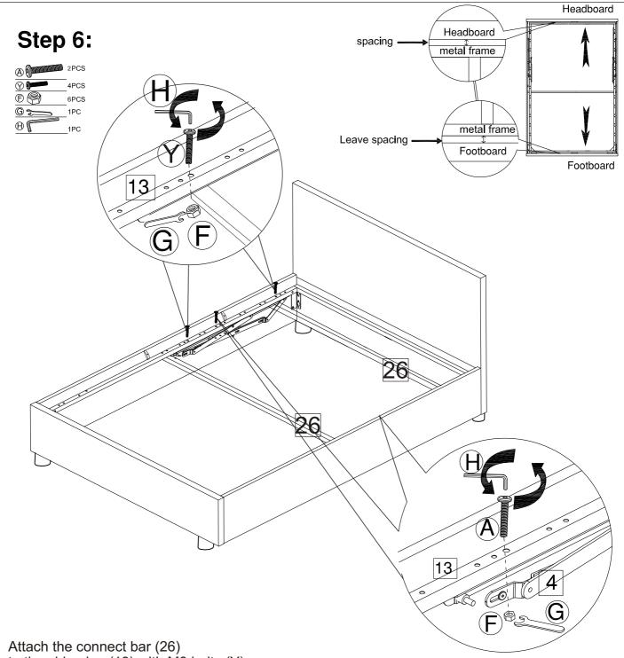
to the side pipe (13) with M8 bolts (Y) and M8 nuts(F) as shown.
