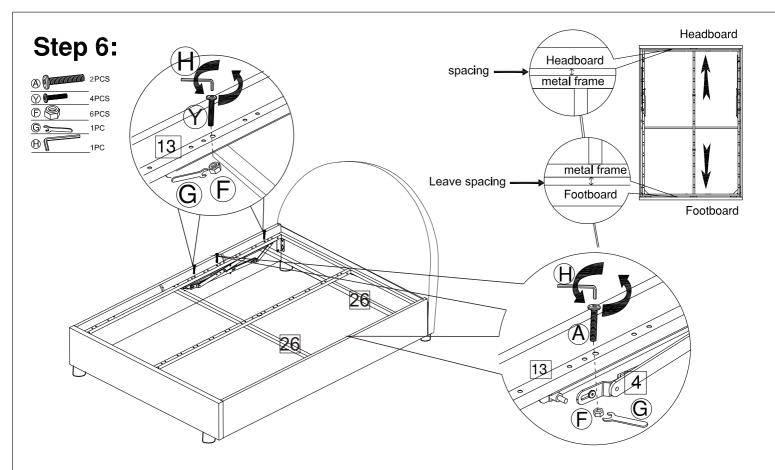
Attach the connect bar (26) to the side pipe (13) with M8 bolts (Y) and M8 nuts(F) as shown.
