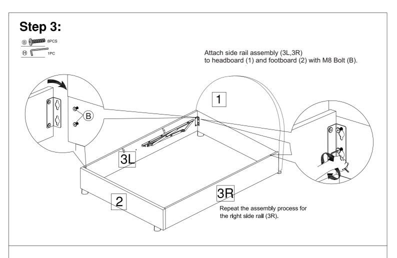
Ensure that the entire bed frame assembly is a regular rectangle as shown below.
