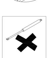
Do not test gas struts by hands, please have them assembled to the metal frame then pull and press the metal base.
