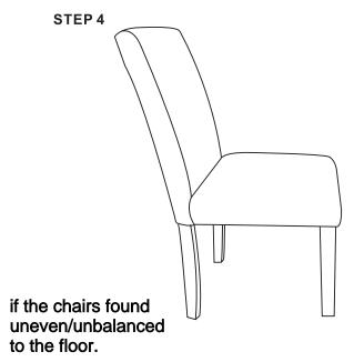
4.please lossen all screws E(80% fixed),and repeat step 2 to check if the chair is alanced to the floor,press the seater if found uneven,then 100% tighten gain
