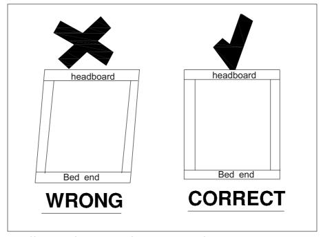
\* gas lift mechanism will be affected if the bed frame is out of shape.
