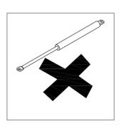
Do not test gas struts by hands, please have them assembled to the metal frame then pull and press the metal base.
