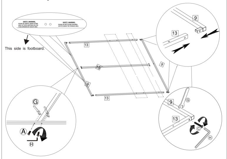
Assemble the interior framework (15 and 9) as shown with M8 bolts (A).
