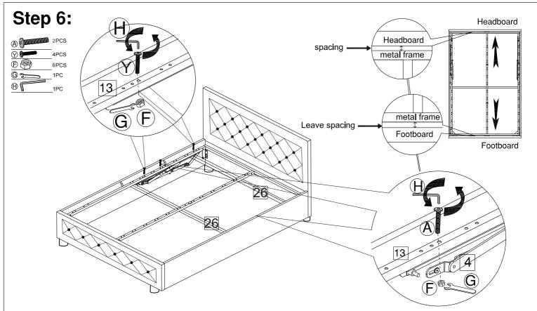
Attach the connect bar (26) to the side pipe (13) with M8 bolts (Y) and M8 nuts(F) as shown.
