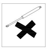
Do not test gas struts by hands, please have them assembled to the metal frame then pull and press the metal base.
